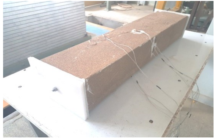
Fig. 13 The aluminum box used as the lining of the tunnel in the second shaking table test
