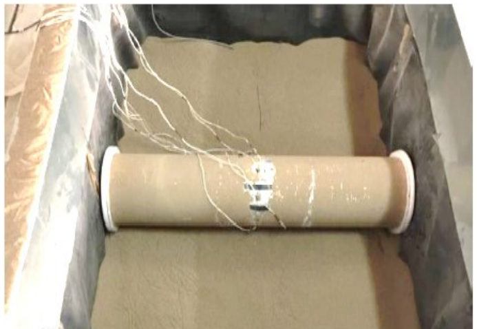
Fig. 7 The used aluminum box to model lining of the circular tunnel
