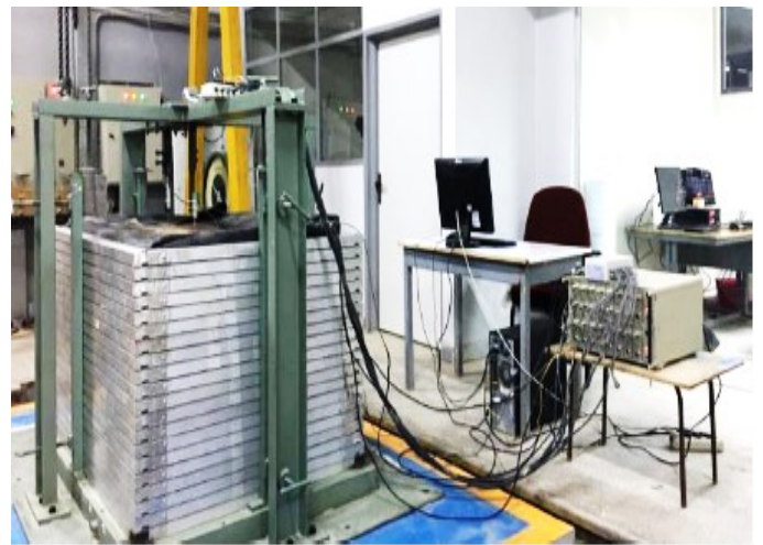
Fig. 6 The shaking table apparatus and the used laminar shear box in experiments
